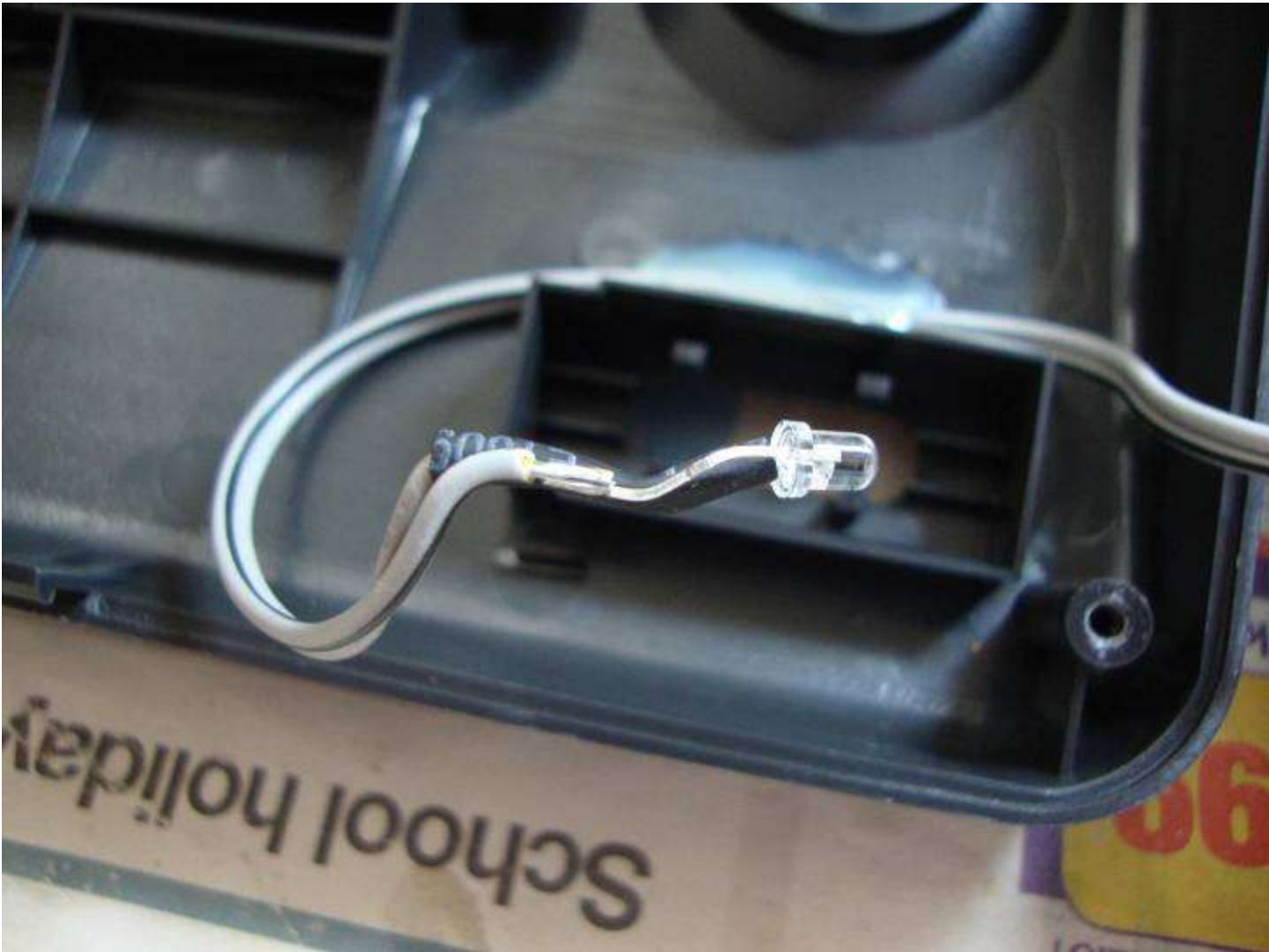
From here fit the switch as shown. The LED needs to be as high in the switch as possible to “throw” the light out of the switch.
